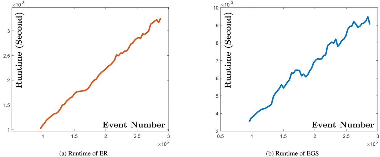
Figure 2. Runtime of ER and EGS computed using the sequence: *focus\_board\_dark\_dynamic*. We randomly sample events in this sequence to generate a subset and measure the computing time of our algorithms in this subset. As we gradually increase the size of the subset, we can see that the runtime of our algorithm is linear to the event number.
